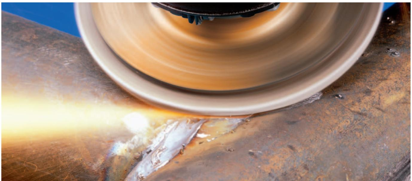
Tool with aggressive stock removal performance and long tool life for demanding multipurpose grinding work.
