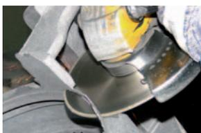
Electroplated diamond cut-off wheels can also be used for cutting off risers, feeders, sprues, parting lines or burrs on grey and nodular cast iron (GG/GGG and GJL/GJS) workpieces. They are characterized by an exceptionally long tool life and an ideal cutting performance when working in deep-laying areas (due to constant tool diameter). In addition, they allow quick and comfortable elimination of burning-in.
