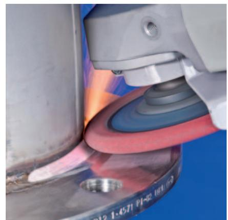
High-performance tool SGP CO-CURVE with high stock removal rates, for demanding grinding work, especially for achieving fine surface finishes.
