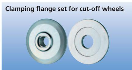
Special flange dia. 76 mm for drive spindles M14 or 5/8" of tool steel. Increases lateral stability and improves power transmission on cut-off wheels.
