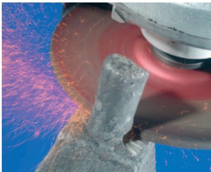
Very hard high-performance tool of hardness T, with outstanding grinding performance and tool life.
